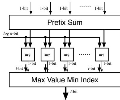
**Figure 9: The index select module and the max value min index module. The index select module is composed by a prefix sum circuit and an array of equality checkers.**
