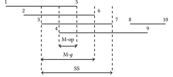
**Figure 7: A five-sensor system with  $M-g$ ,  $M-op$  and  $SS$ .** The sensor input intervals are  $[1, 5]$ ,  $[2, 6]$ ,  $[3, 7]$ ,  $[4, 9]$ ,  $[8, 10]$ . The resulting intervals are  $[3, 6]$ ,  $[4, 5]$ , and  $[3, 7]$  for  $M-g$ ,  $M-op$ , and  $SS$ , respectively.
