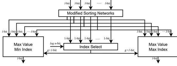
**Figure 6: The complete circuit design for  $M-g-U$ .**  $n$  is the number of sensors,  $l$  is the length of the endpoint of the input interval, and  $g$  is the number of faulty sensors. There are  $2n$   $l$ -bit inputs for the circuit.
