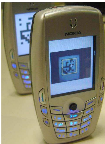
Figure 4. SiB application on a Nokia 6620 with one phone scanning the hash-barcode on the LCD of another.
